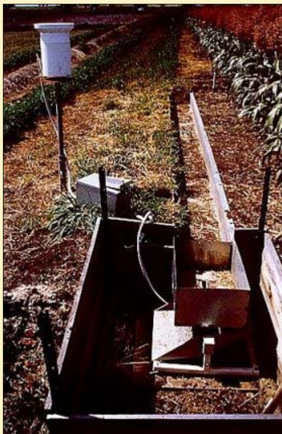
Trough and equipment used to measure surface runoff from an experimental plot planted to sorghum
